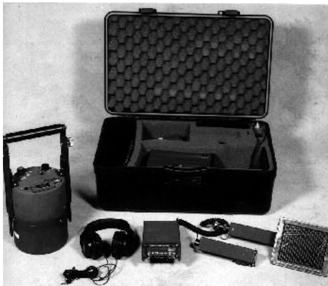
Figure 7-C: AN/PDR-77 with case on left. All the probes, including those from the extension kit, are on the right.
