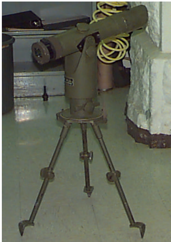
Figure 3-A: M1A1 Infinity Collimator (contains 10 Ci of Tritium)
