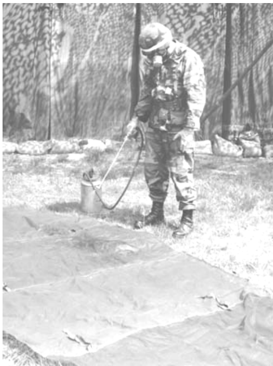
Figure 2-23. Applying Permethrin by 2-Gallon Sprayer to Insect Net Protector (Mosquito Bed Net)
